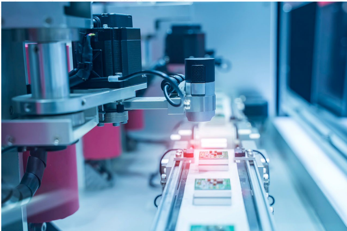
Figure 1: Robotic vision sensor camera system in a smart PCB factory.
